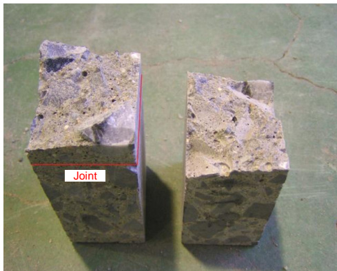
State of damage on other than joint surface
