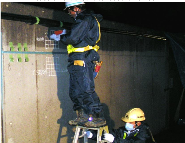
Measurement of surface tensile strength
