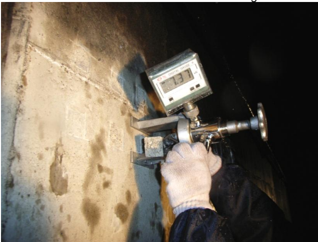
Measurement of surface tensile strength
