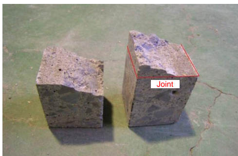
State of damage on other than joint surface
